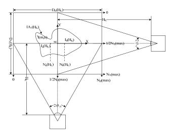
Fig. 6 Measurement of the maximal vertical distance  $D_V(H_K)$ .
