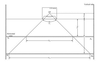
Fig. 7 Mechanism for obtaining an accurate  $h_0$  for a CCD camera.
