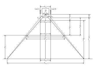
Fig. 2 Schematic diagram illustrating the parallel measuring method.
